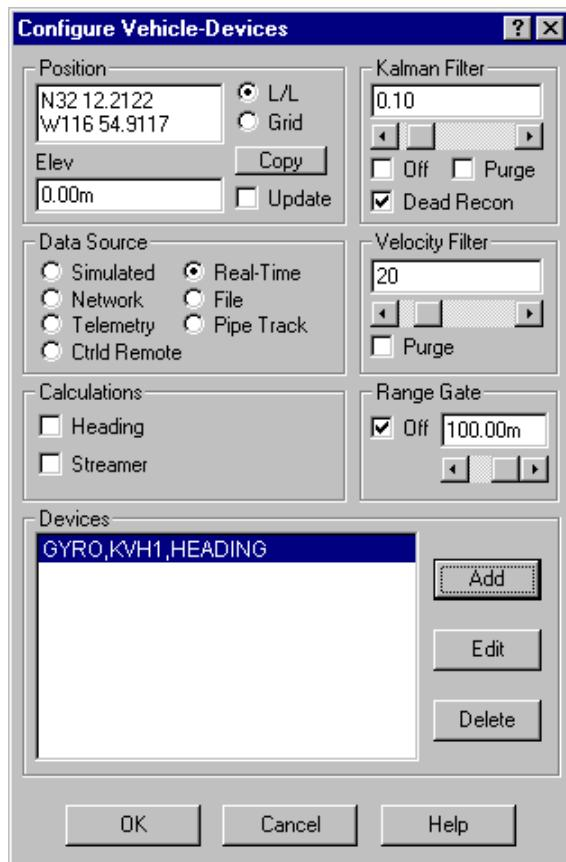
Once the KVH Gyro device has been added to the vehicle, it must be configured to suit the vehicle and application. Highlight the Gyro, KVH1, Heading device and click the Edit button. The Configure Gyro dialog box appears, as seen below.
